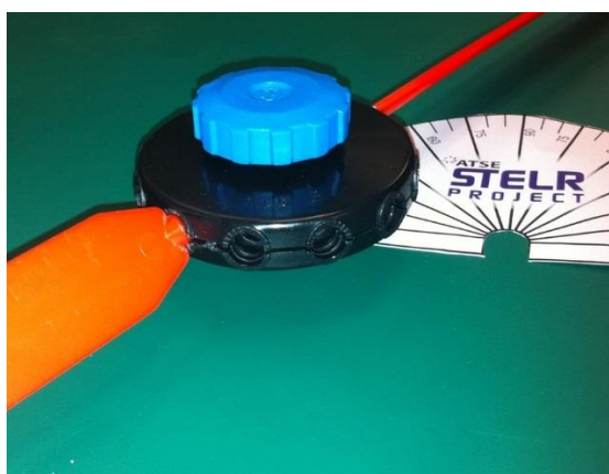
Figure 2: These blades have been set into the hub at the same angle (45°)
