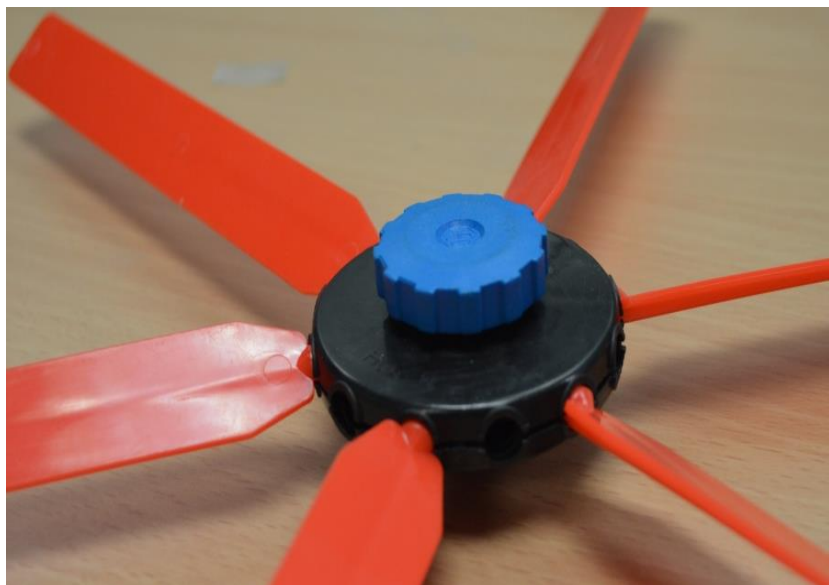
Figure 3: These blades have been set into the hub at the same angle ( 45^\circ )
