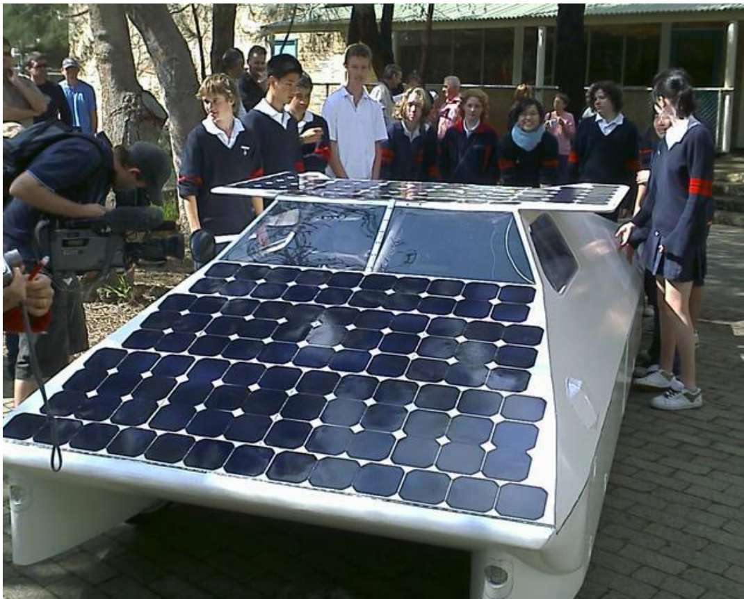
Figure 4: The solar cells on the Willetton SHS solar car are connected in series and parallel to give a desired DC voltage.
