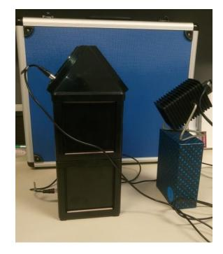
Once this is set up and the probes are connected to the data logger run the logger for 20 minutes without the light being turned on.
