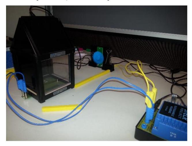
For each the data logger ran for 40 minutes. The results were then downloaded to a computer. From the spreadsheet the data was reduced, deleting rows, to measurements taken every 30 seconds. These results are given below. Temp 1 being the ground floor temperature and temp 2 being the attic temperature.
