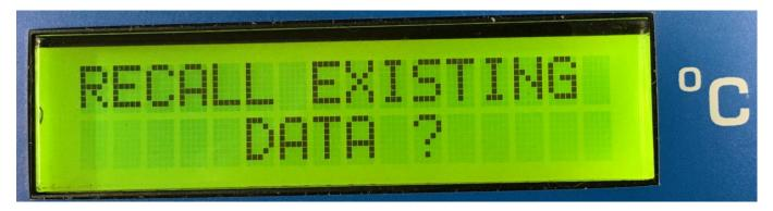
6. Next choose the time interval for taking readings. Use the up or down arrow buttons to change the interval. You can choose between 1 sec, 3 sec, 15 sec, or 60 sec. Press the "ENTER" button when you have the time interval you want.
