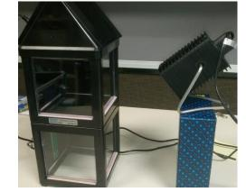
Note – the level dividers are black plastic, no insulation is used and there are two windows on each floor.
